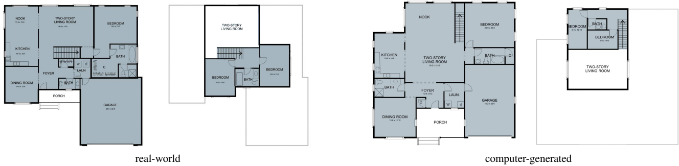
Figure 11: A two-story layout designed by an architect (left) and an automatically generated layout for the same architectural program (right).
