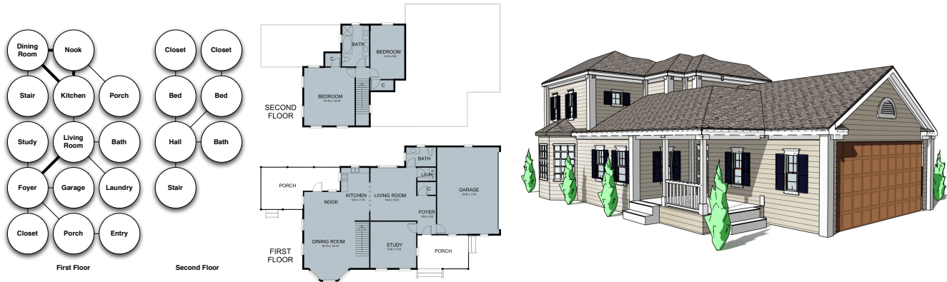
Figure 1: Computer-generated building layout. An architectural program, illustrated by a bubble diagram (left), generated by a Bayesian network trained on real-world data. A set of floor plans (middle), optimized for the architectural program. A 3D model (right), generated from the floor plans and decorated in cottage style.
